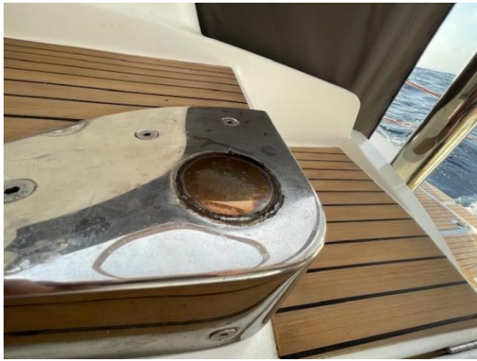
(Fig2: Base plate following failure)
